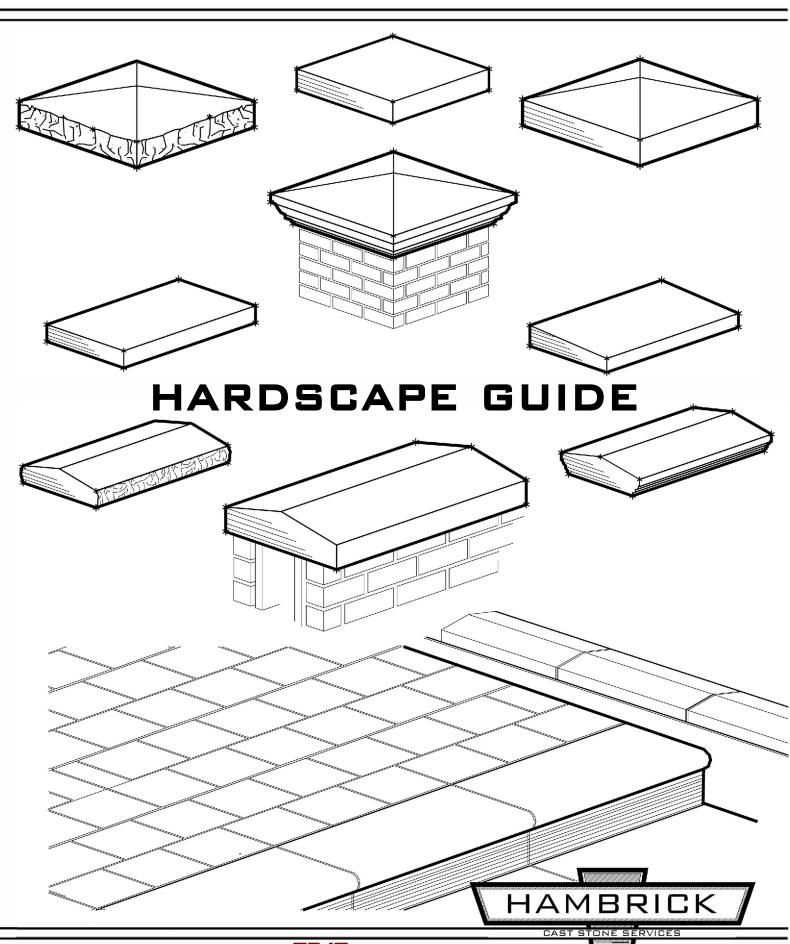
Pier caps are made in sizes to cover standard masonry piers, with a  $\frac{1}{2}$ " to 1" overhang on each edge. Although most pier caps are square, custom rectangular or special angled caps are available by special order.
